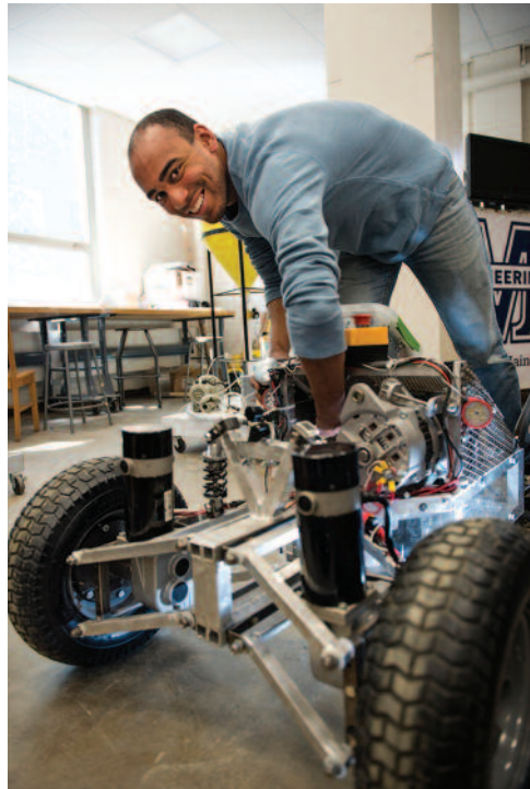
Mechanical engineering students are designing, building, and testing fully autonomous land drones that can traverse unstable, muddy terrain and navigate using GPS.
